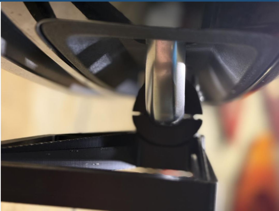
Figure 6. Side view of the installed clamp showing the remaining gap between the front and rear retention brackets.
