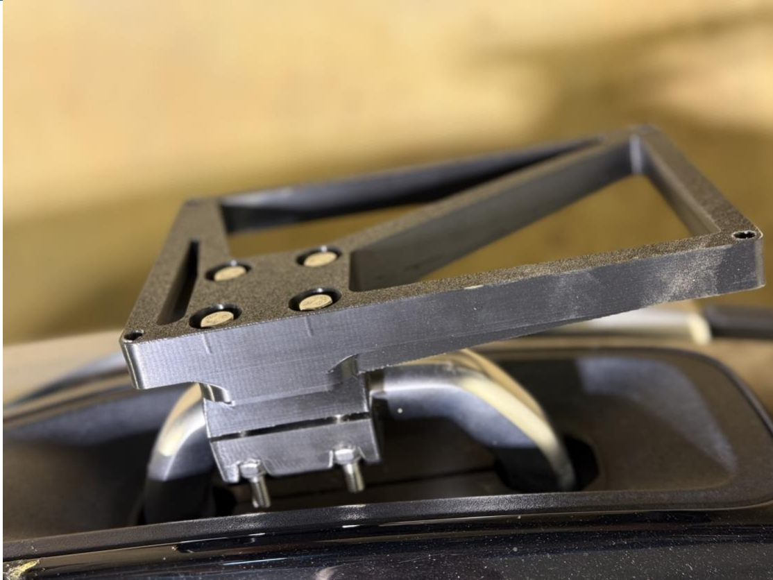
Figure 9. Installed tow-hook plate mount shown after final adjustment.
