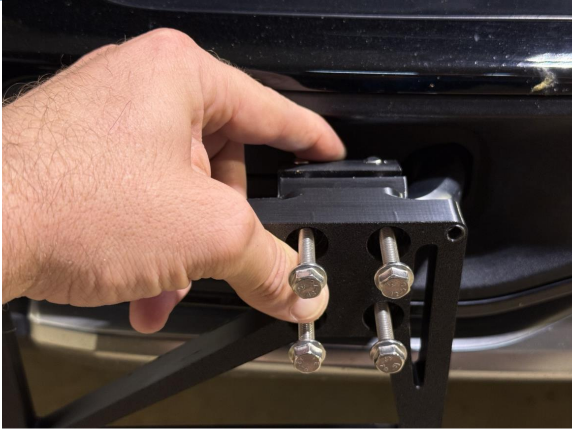
Figure 5. M6 screws engaged with the captured lock nuts in the rear retention bracket.
