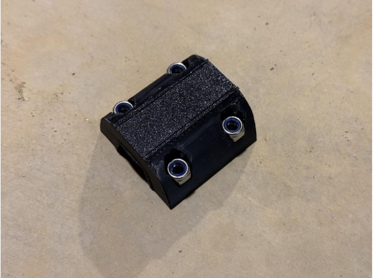
Figure 1. Four lock nuts fully seated in the rear retention bracket with the blue nylon rings facing outward.
