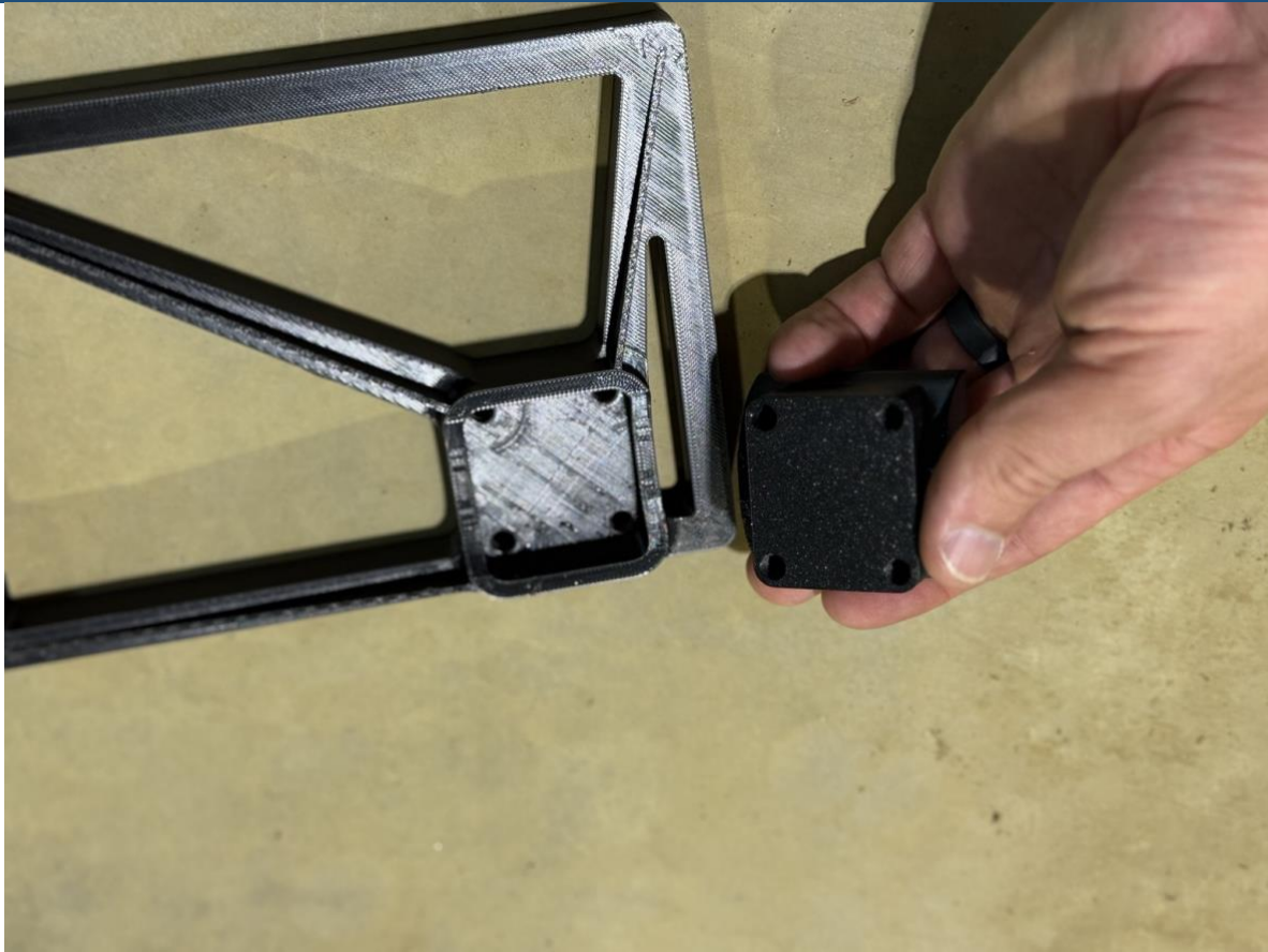
Figure 3. Front retention bracket aligned with the rectangular opening and rounded profiles matched.
