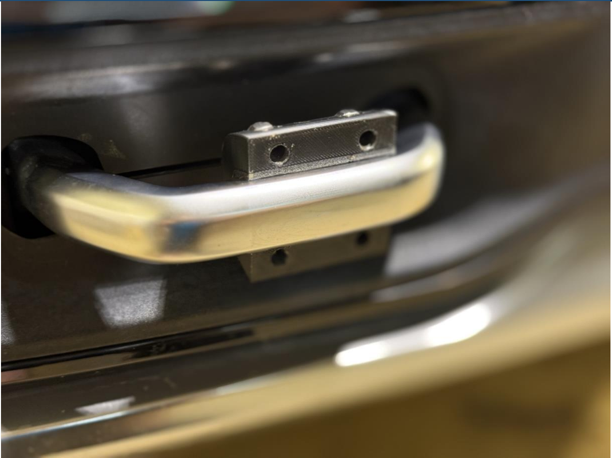
Figure 2. Rear retention bracket positioned on the passenger-side tow hook and shifted toward the driver side.
